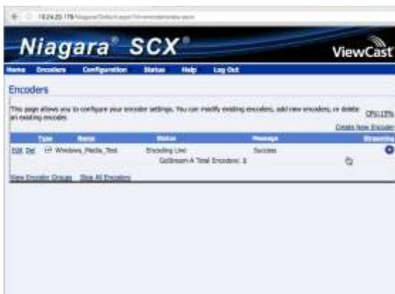
Now we want to view the output stream. For this example we are using Windows Media Player to connect from a desktop computer on the same network as the encoder.
